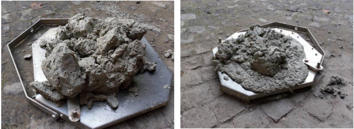
Figure 2. Same sample of soil before and after the addition of foam
